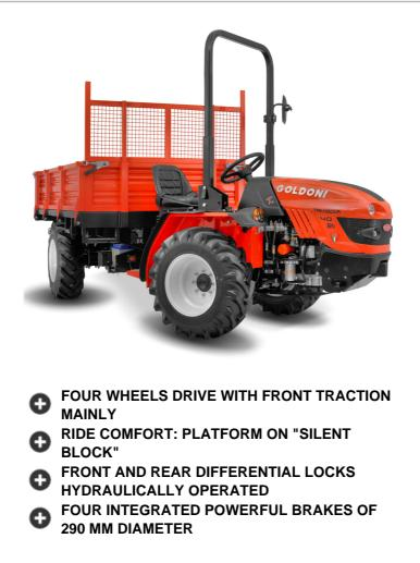
Goldoni T range has been designed to meet the specific needs of people who work in mountainous areas and require a machine that's particularly suitable for materials handling. With or water cooled engines to choose from, steering wheels or articulated versions, 2 homologated versions available such as agricultural tractor or as utility vehicle.
